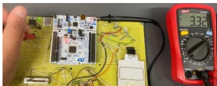
Figure 20: 3.3V regulator test
