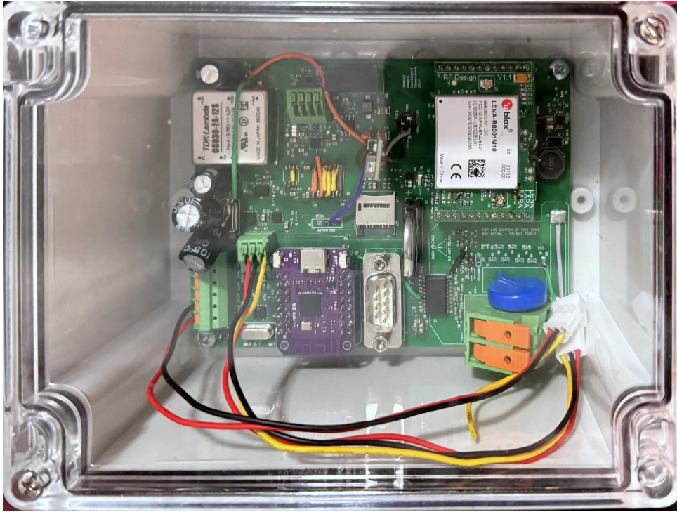
Figure 4.22: Fully assembled enclosure with the mounted PCB.
