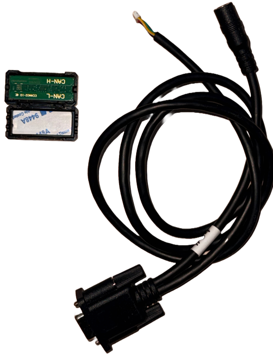
Figure 3.12: Clip-on CAN inductive probe and interface cable for non-intrusive signal tapping.
