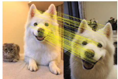
(b) Matched Features Following Lowes Ratio Test. Reproduced from [32]
